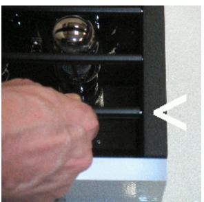
To complete the installation, press the bar in the direction of the pin already inserted, and manoeuvre the other end into the corresponding dimple in the other side rail. In this illustration, the bar is pressed to the left, while the right spring pin is set into the dimple in the right side rail.
