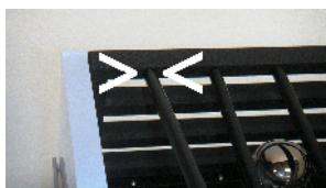
The top tube cage bars have a spring pin in each end. To install, place one of the spring pins into one of the small dimples machined into one of the side rails. In the illustration, the pin has been located into the left side rail.
