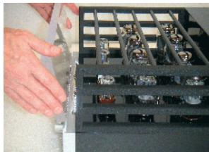
The glass installs in the groove at the top of the fascia. Insert it at a slight angle, as shown. Handle the acrylic glass carefully, and do not scratch it. Scratches will show strongly when the panel is lighted in normal operation. Your panel was carefully inspected prior to packing.
