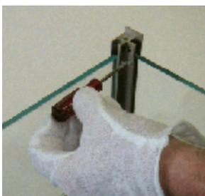
Tighten the four white nylon setscrews that secure the front glass using the tool provided. Turn clockwise to tighten.
