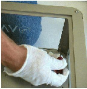
The front glass has the etched VAC logo. Install this between the front pillars.
