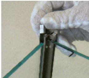
Install the six aluminum blocks at the top of the rear glass and side glasses. If there is a 'dimple' in the block, it should face the outside of the amplifier.
