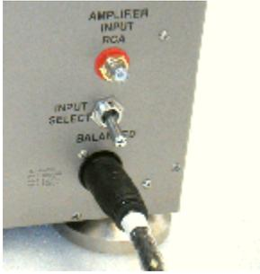
XLR connection, balanced or single-ended, are made to the XLR jack on the rear panel.
