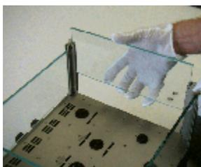
Slide the side and rear glass plates into the pillars' channels. Note that the rear glass is slightly wider than the side glasses. The glass will not go all the way to the chassis top, but has a gap at the bottom for air flow. Take care not to scratch or break the glass.
